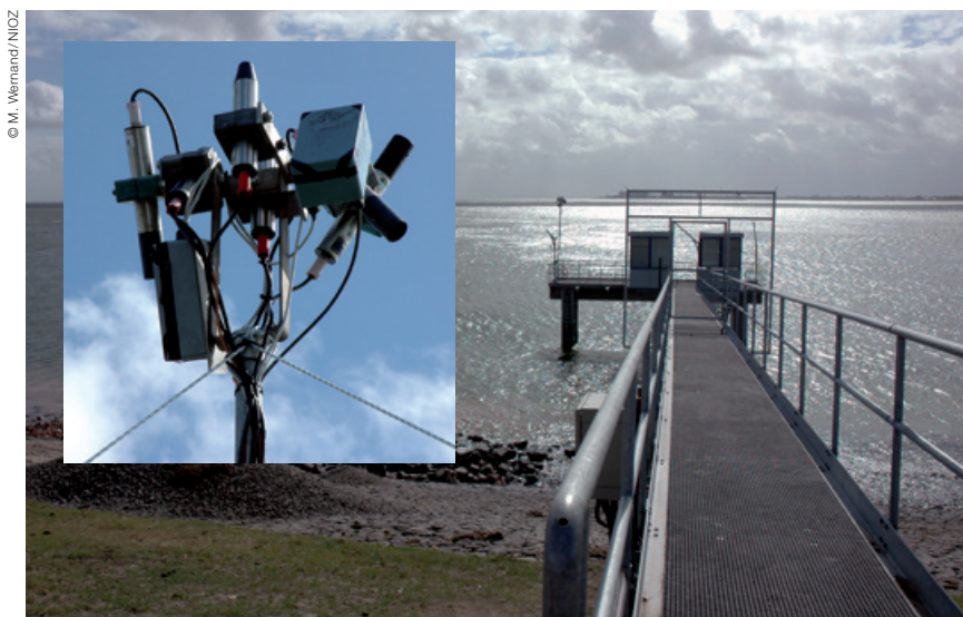
Figure 8: In situ sensors on NIOZ (NL) jetty, two looking to the sky measuring the spectral radiance L_{sky} between 350 and 950 nm (for all sensors except UV), one measuring incoming sunlight E_s , one measuring incoming UV-sunlight E_s (280-580nm) and two looking to the sea water measuring the spectral radiance L_{sc} (surface radiance)
