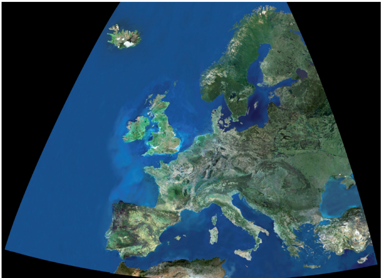
Figure 2: Approximately 160 separate MERIS images make up this mosaic of Europe. The images were acquired by MERIS, then georeferenced, colour-matched, clouds masked out with cloud-free data, and built into a single image.
