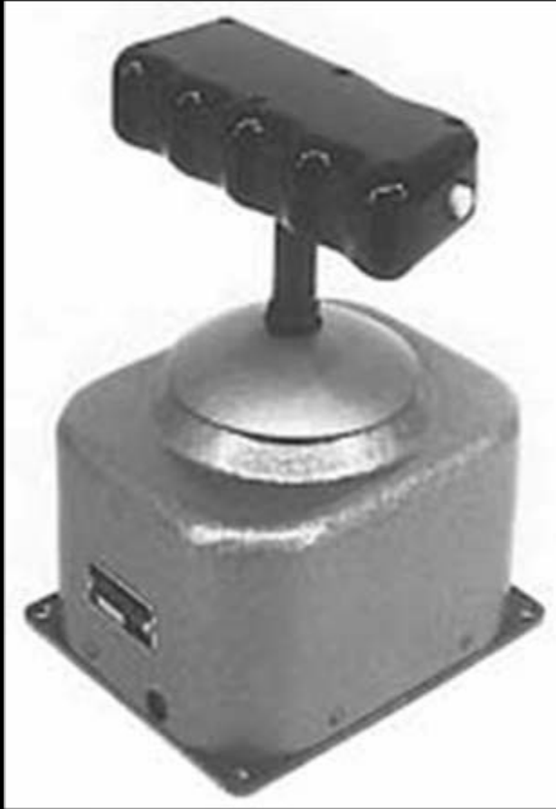
Gagarin's hand controller, designed by "artillerymen"
