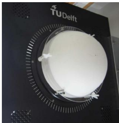
Fig. 4.1. Hemispherical dielectric lens fed by an array of connected slots built at the Technical University of Delft.
