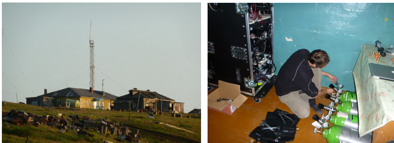
Figure 2: Left: the Ambarchik weather station with the newly erected tower. Right: the author installing the calibration gas tanks. In the background: the rack harboring the Picarro analyzer, data logger, air flow control system, etc. Image courtesy of M. Hertel.
