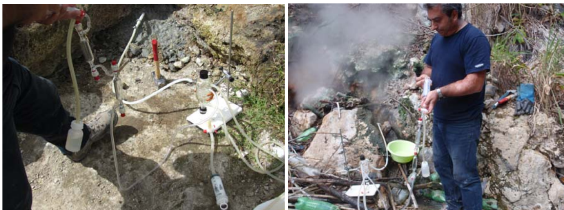
Fig. 4 Sampling of fumarolic fluids.
