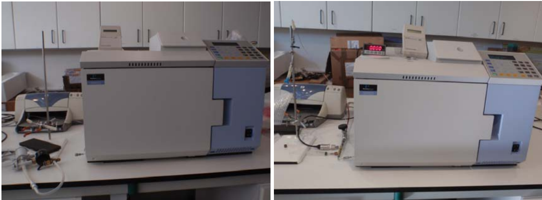
Fig. 1 a) original setup of GC where the vacuum was done by means of a manual pump b) Implementation of the GC with a vacuum gas line and a control of the injection pressure.
