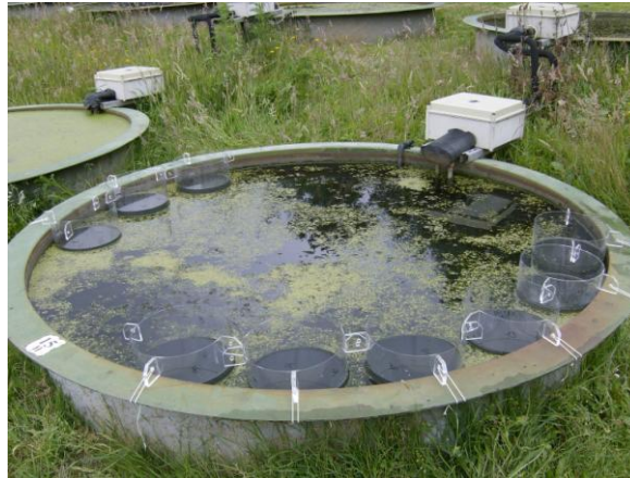
Fig. 1: 20L enclosures installed in a high temperature mesocosm
