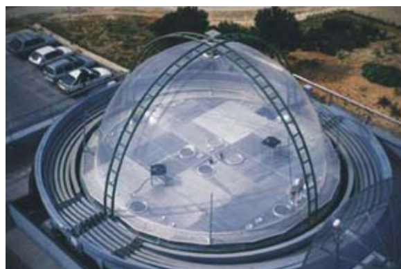
One of the two identical EUPHORE reactors in Valencia, Spain. Each of them consists of a hemisphere with a diameter of 9.2m and a volume of 200 m 3 . Photo: CEAM Valencia
