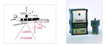
Figure 1: Airborne laser scanning system components, schematic illustration (left) and laser scanning device (right).
